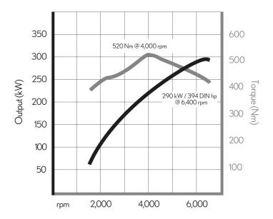
The 4,969cc V8 is derived from the 4.6-litre unit which powers the Lexus LS 460, with the stroke extended by 6.5mm to 89.5mm – intended to just reach the design limit – and the bore unchanged. As well as the increase in capacity, the 5.0-litre engine has undergone significant component modification to handle the greater power output, accommodate the hybrid system and minimise emissions.
