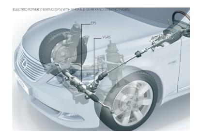
The new EPS is designed specifically for the LS 600h's front multilink suspension design and 19-inch tyres. It has a newly developed step-up DC-DC power converter that increases output from 27 to 46 volts and a bespoke, 110mm diameter high-output brushless motor. Assembled with high precision, the smooth running motor has approximately double the output capacity of a conventional power steering unit.
