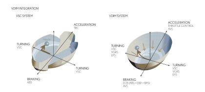
The Driving Response and Acceleration Management System is unique to the LS 600h, giving VDIM unprecedented interaction with both engine and transmission. This employs engine and electric motor output control to effect a faster, smoother and more precise response to situations where there is a risk of loss of traction, such as unwanted mid-corner gear changes.
