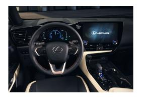
An example of the intuitive control that's central to the concept is the touch-tracer switches on the steering wheel, which can be customised to operate the driver's preferred functions. When the switch is used, its shape is shown on the head-up display, so the driver doesn't have to look down at the wheel to check the function they want to operate.
