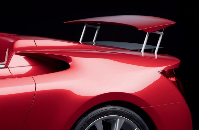
Large intakes ducting cooling air to the rear brakes and rear-mounted radiators dominate the LF-A Roadster profile, and include prominent, high-level, 'turn-up' style intakes informed by the sophisticated, wind-tunnel honed aerodynamics of single-seat racing cars.
